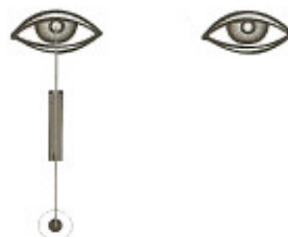
the origin of the line of sight must lie in the center of the pupil of one eye
