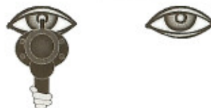
the origin of the line of sight must lie in the center of the pupil of one eye
